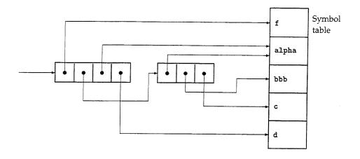
Figure 7.2 Internal representation of the term f(alpha(bbb,c),alpha,d).
