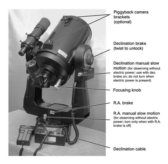
Figure 10.1: Important parts of an LX200 telescope.
