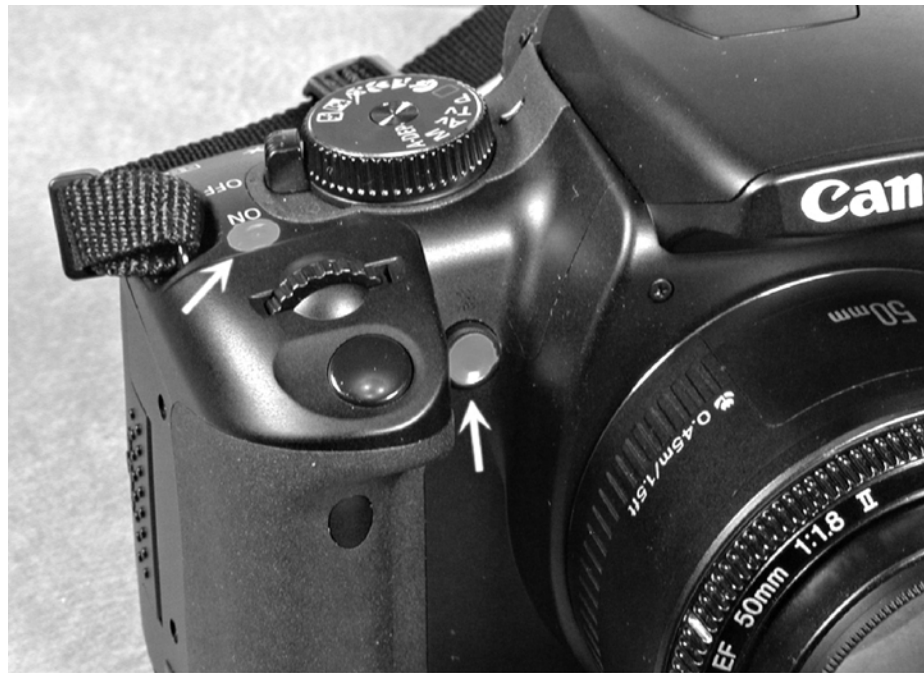
Figure 3.6. Dots punched out of red vinyl tape make good covers for the power-on LED and self-timer indicator.
