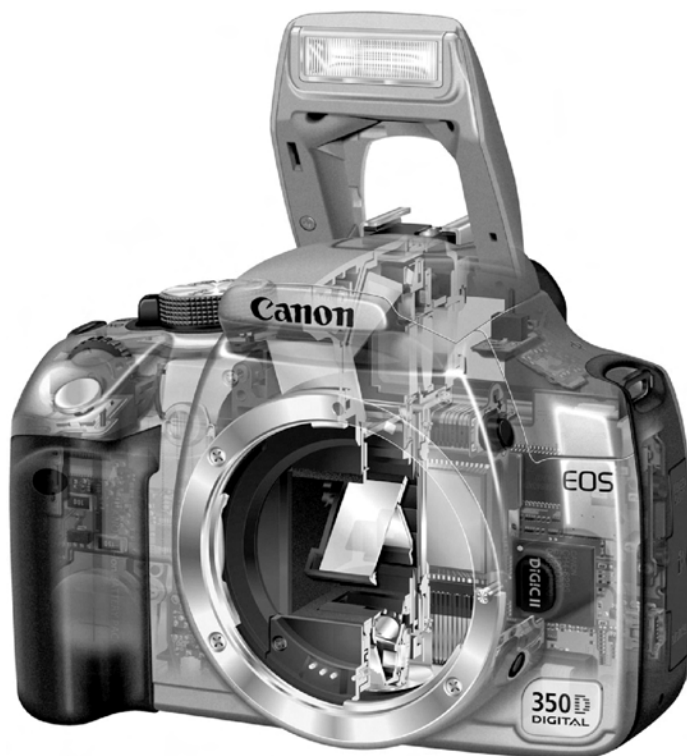
Figure 1.3. A more elaborate view of what's inside a DSLR. Note computer circuitry ("DIGIC II") at right. (Canon USA.)
