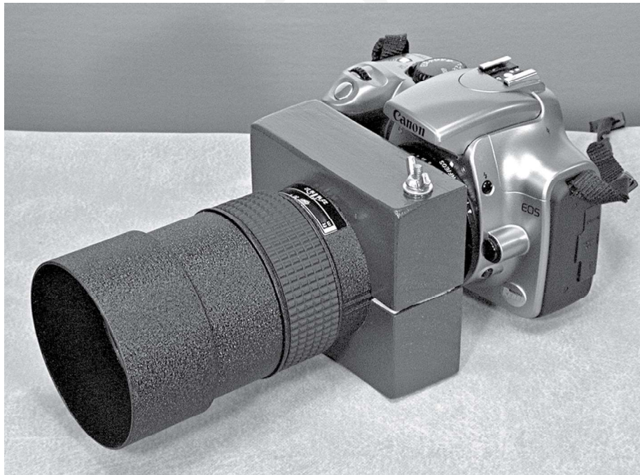
Figure 7.11. Homemade tripod collar for Nikon 180/2.8 AF lens consists of wooden block with large round hole, slot and bolt to allow tightening, and a 1/4"-20 threaded insert on the underside.
