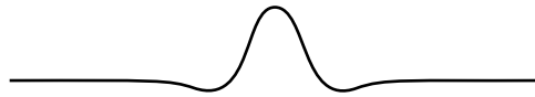
Figure 13.9: A wavelet (one of many types). A complex signal can be described as the sum of wavelets.
